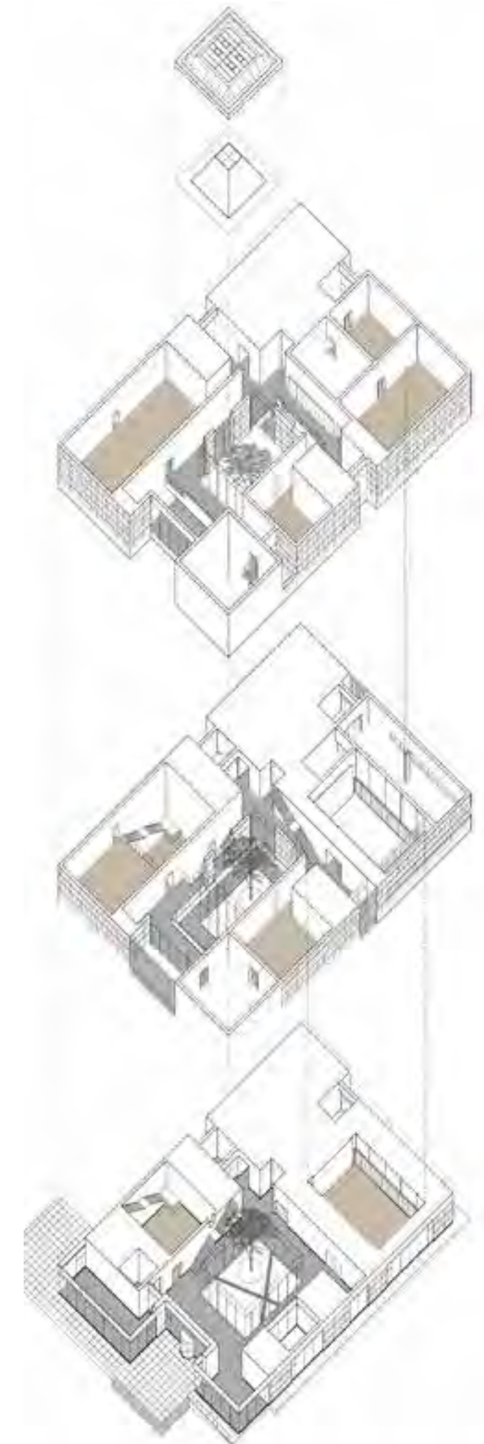
Final distribution of the public areas on the three main floors. Access and ancillary spaces (gray), exhibition areas (brown).
